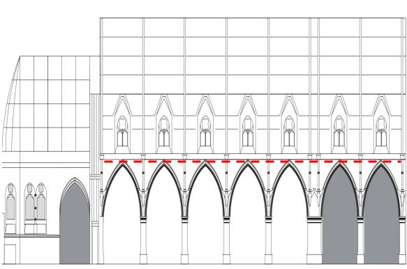
Existing wiring that enters Aisle at high level is in good condition and will be utilised. At this point, new wiring will be connected and extended along the Aisle horizontal beam at the apex of the roof following the existing wiring route.
